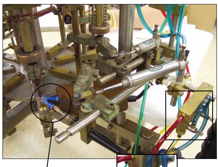
The machine consists of a rotating center carousel with eight stations. The individual components of each slip-on fitting are loaded into clamp fixtures mounted on the carousel. The carousel indexes to each of the process stations: load, heat, cool, quench, and unload. The control and timing of the machine is accomplished using Clippard modular valves and brass limit
